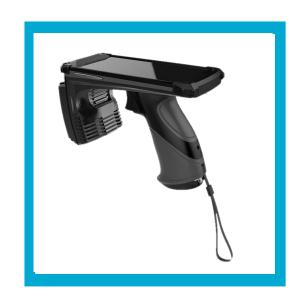
Orca-50-Air UHF handheld data terminal offers optimal performance and excellent multi-tag identification ability. Orca-50-Air offers a lightweight, elegant and compact design, featuring a large 5.00" LCD screen. It uses industrial and military grade components to ensure stability and endurance in harsh environments, with excellent drop protection. Its pistol style hot swapping battery system makes backup battery more convenient to be restored, so that the operating time is unlimited.
