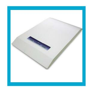
The specific antenna design combined with an integrated motion sensor provides a very good reading zone containment, making it possible to use SPU-500 in confined environments. Thanks to its embedded intelligence, SPU500 is able to detect moving as well as static items.
